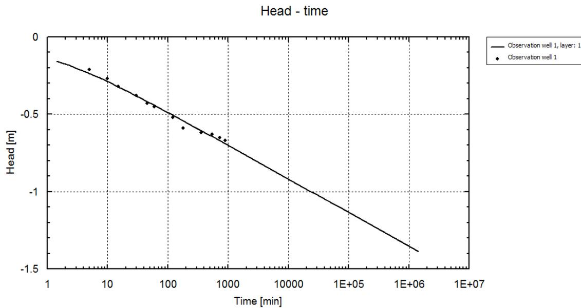
Figure 5: Time-drawdown curve from Kwale pump test.
