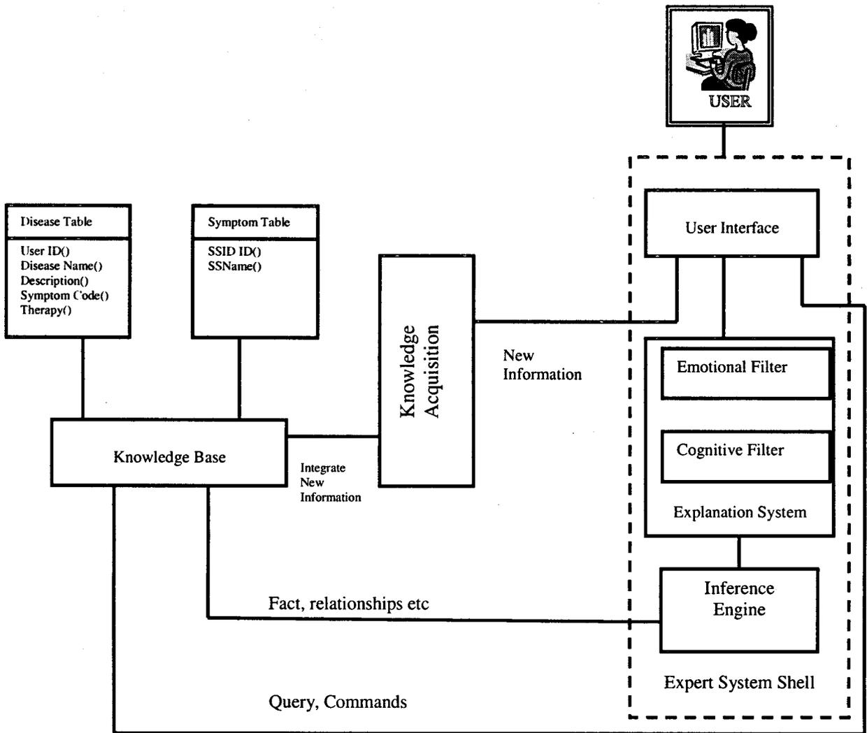
Figure 3: Conceptual Diagram of the Medical Expert System
