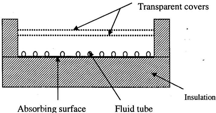
**Fig. 3 Basic Flat Plate Solar Collector**
