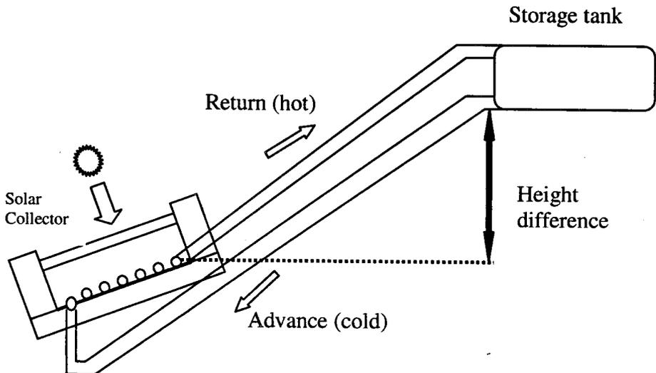
**Fig. 1 Schematic Diagram of a Thermo-siphon System**
