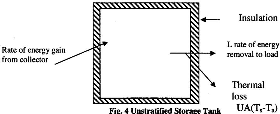
Fig. 4 Unstratified Storage Tank
