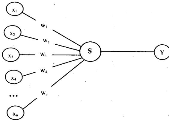
**Figure 1.** Simple structure of Artificial Neural Network.
