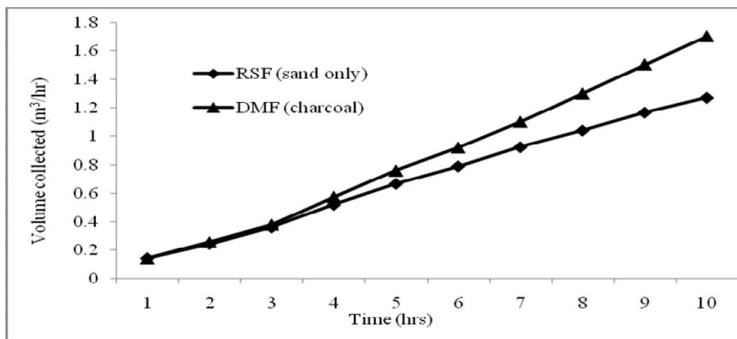
Fig. 11: Variation of the volume of water collected versus time (90-110 FTU)
