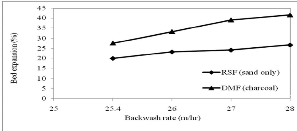
Fig. 9: Variation of bed expansion with backwash rate
