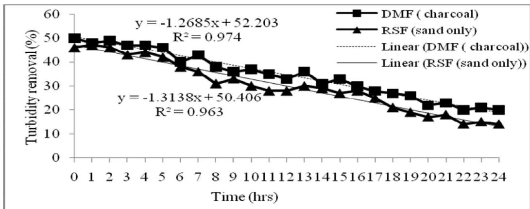
Fig. 5: Variation of turbidity removal with time, filter depth 60cm
