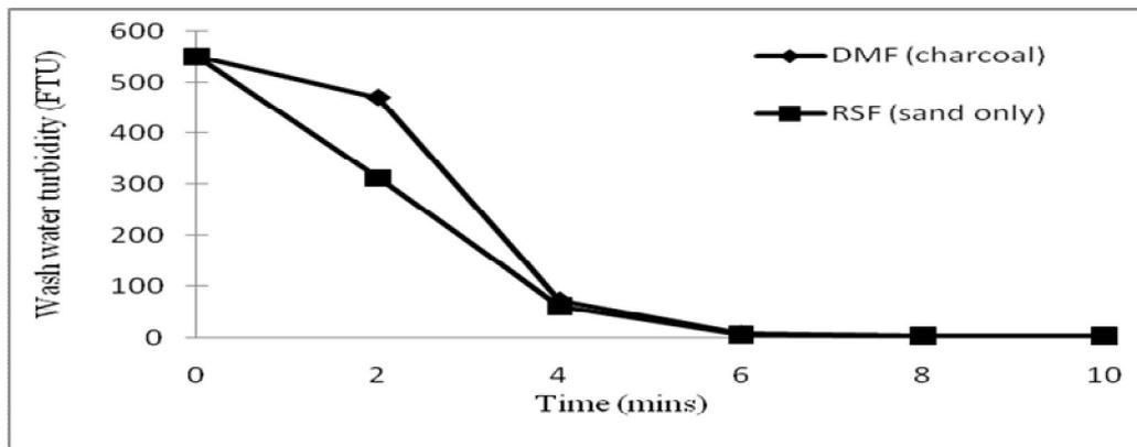
Fig. 8: Wash water turbidity versus time (kaolin)
