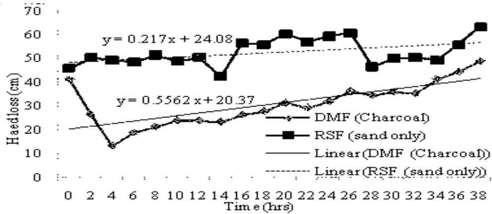
Fig. 6: Variation of total head loss with time (kaolin)
