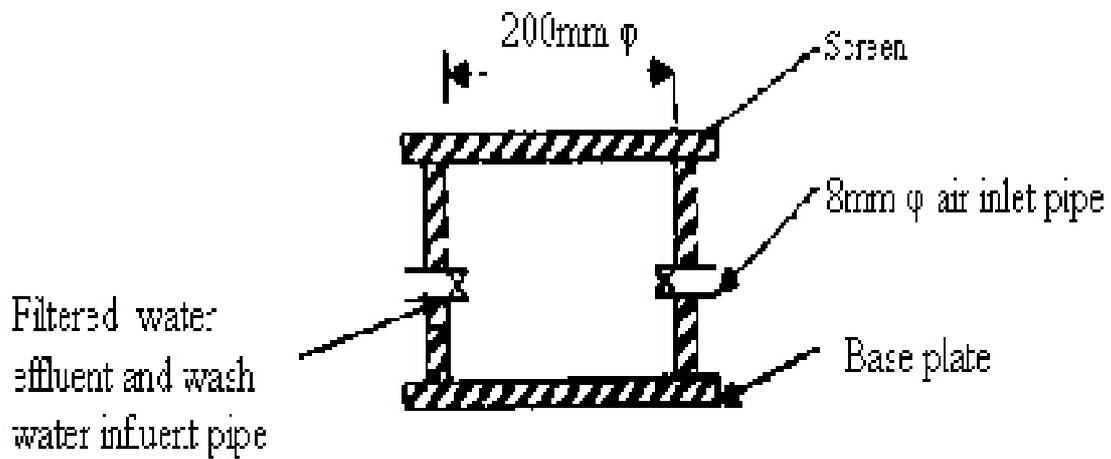
Fig. 2: Schematic representation of the base (underdrain)
