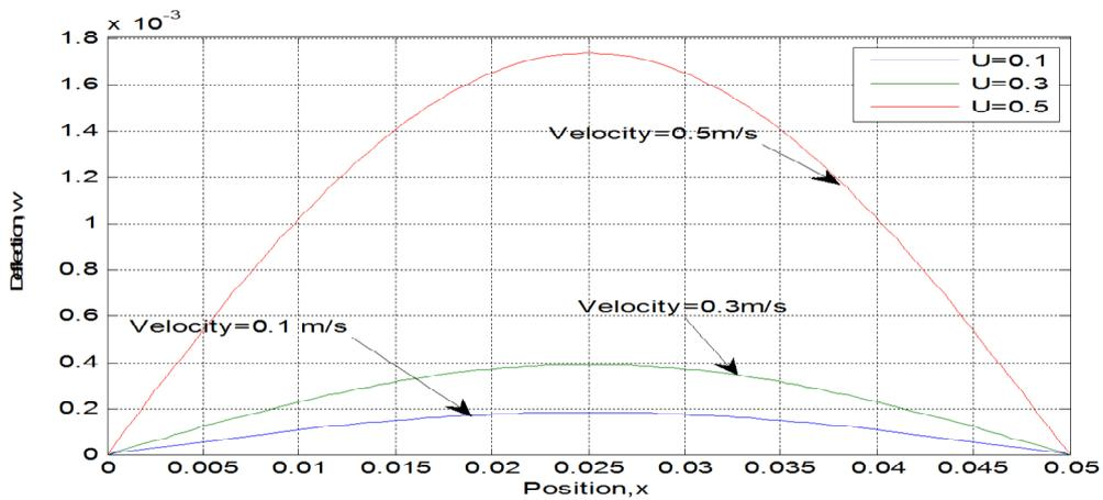
Figure 7: Plot of Response  $w$  versus Position for Varying Velocity for MAP=93 mmHg
