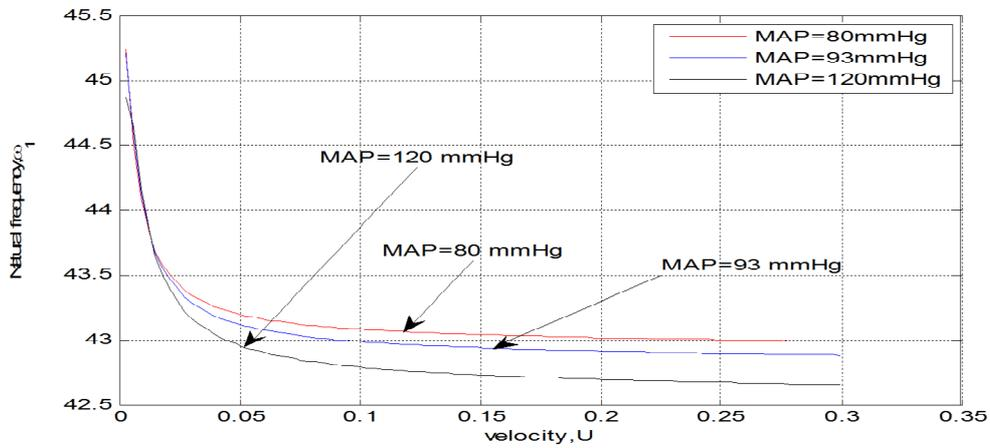
Figure 4: Plot of Primary Natural Frequency  $\omega_1$  versus Velocity for Varying MAP Values
