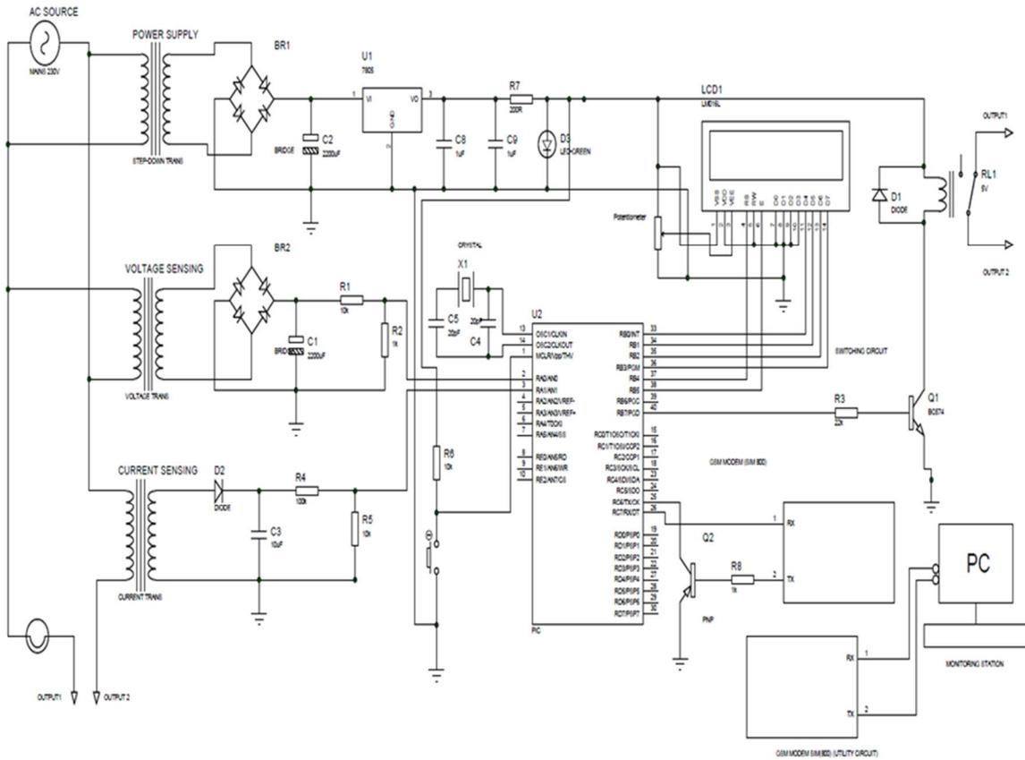
Figure 3: Complete Schematic diagram for AEMS\_GSM
