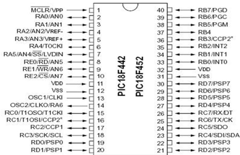
**Figure 6: PIC18F452 microcontroller Pin Configuration**
