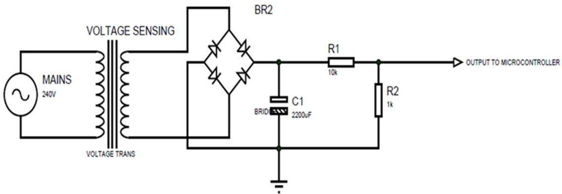
Figure 4: Voltage sensing circuit
