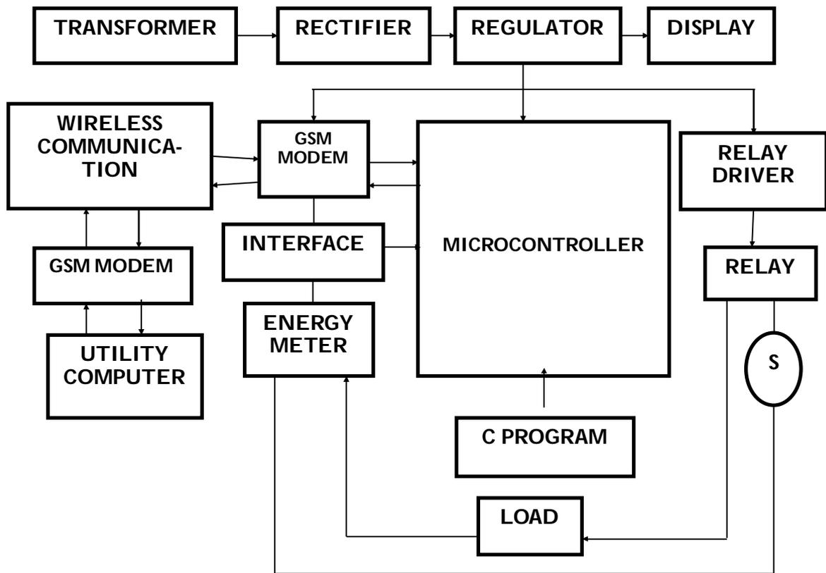
**Figure 2: Functional block diagram of the AEMS\_GSM**
