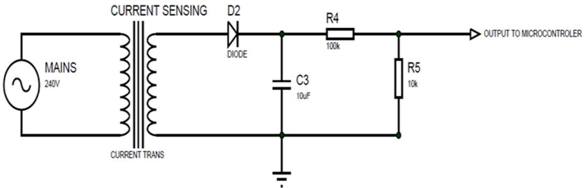
**Figure 5: Current sensing circuit**
